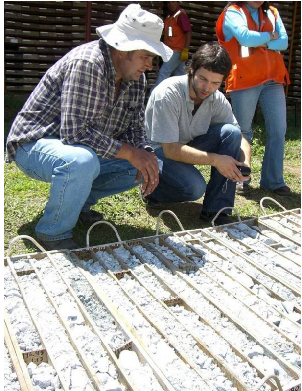
Heavily broken cores to scan and analyse
