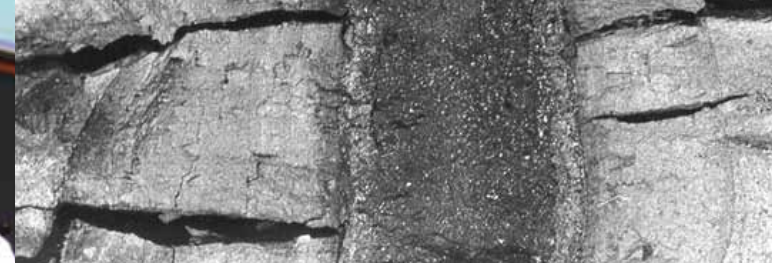
Coke oven charge after half of coking time
