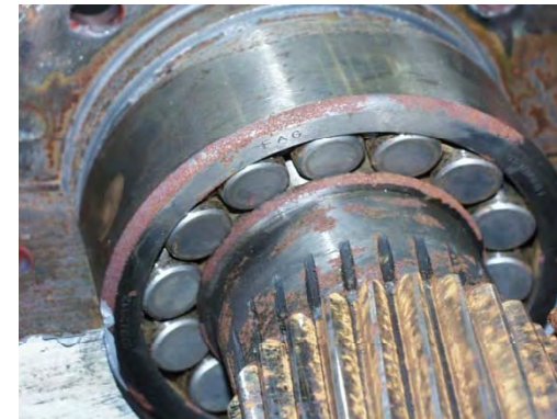
Tooth flank corrosion
