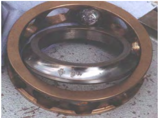
Bearing wear damage
