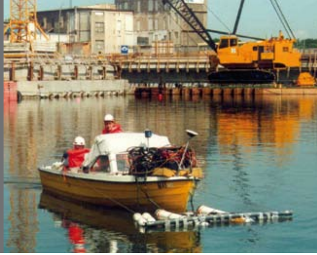
Hydroacoustic measurements for site investigation in Berlin
