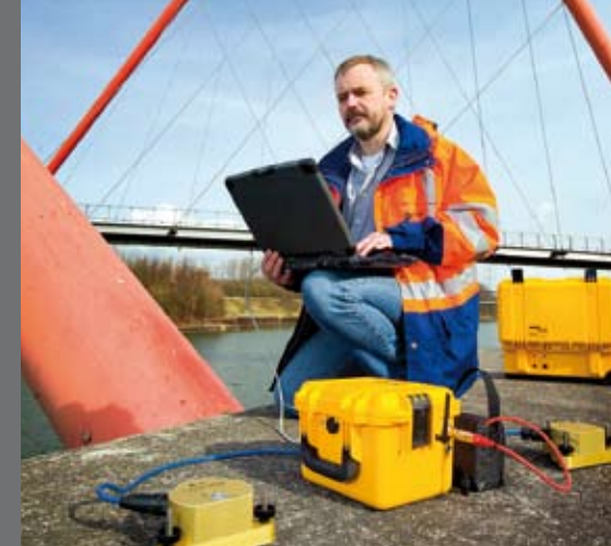
Vibration monitoring at a bridge foundation
