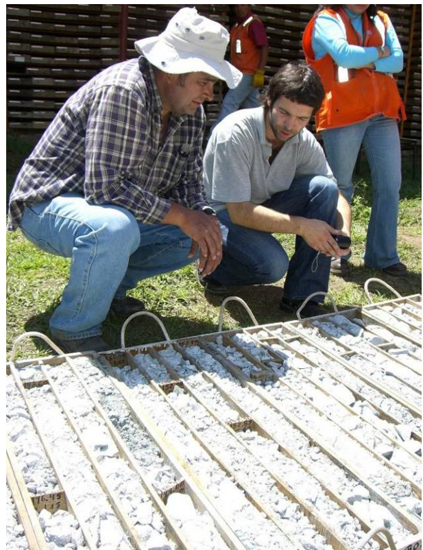
Heavily broken cores to scan and analyse
