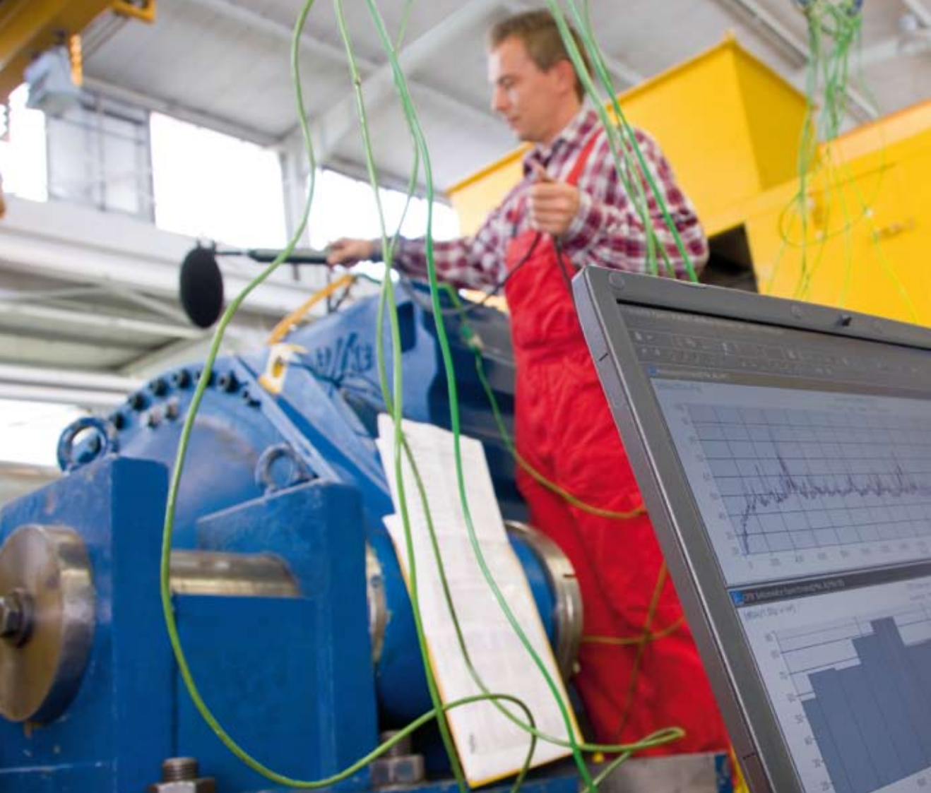
Noise generation by a wind turbine transmission is examined at the DMT test facility to determine compliance with specifications.
